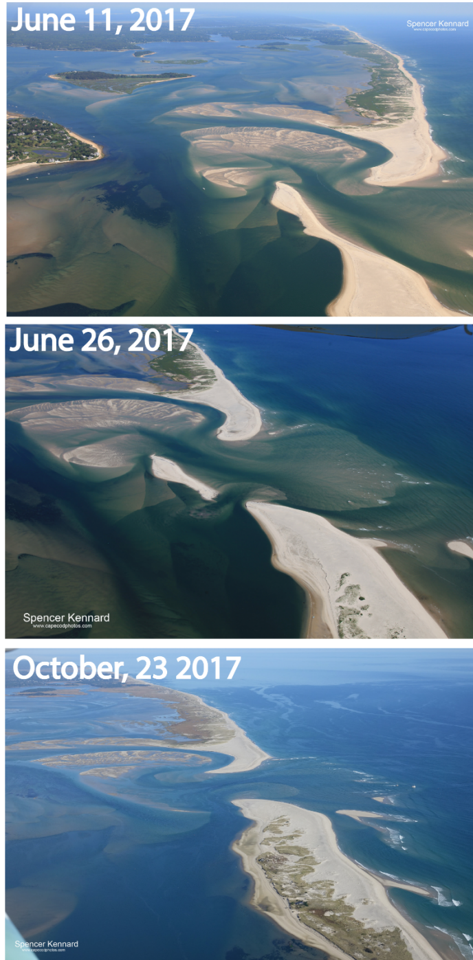
Figure 10. Aerial photographs showing changes in configuration of North Inlet between June and October, 2017. The breakup of the NW-trending spit on northern North Beach Island made way for a more efficient ebb tidal channel along the southern margin of the North Inlet complex of shoals and channels (courtesy of T. Keon).
