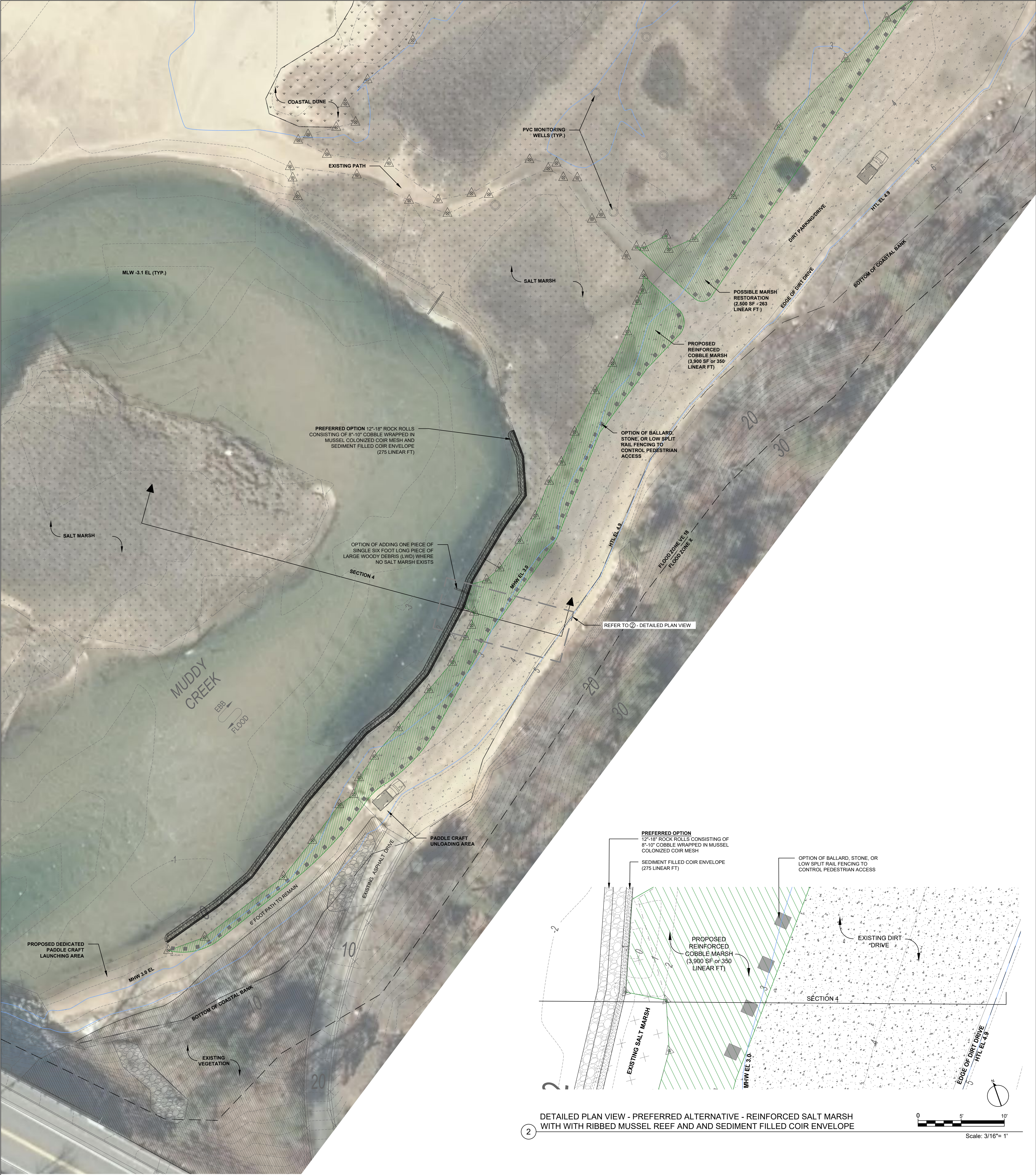
1 RESTORATION PLAN - PREFERRED OPTION - LIVING SHORELINE ALTERNATIVE C - COBBLE REINFORCED MARSH WITH RIBBED MUSSEL REEF 0 20' 40' Scale: 1"= 20'
