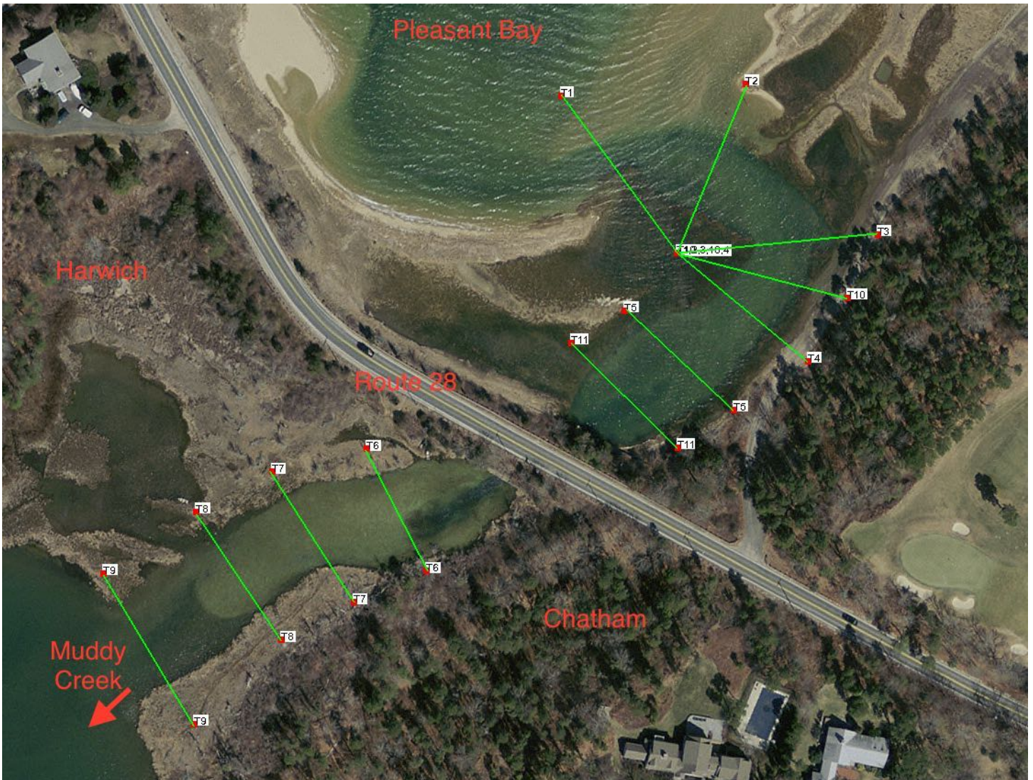
Figure 7: Chanel bathymetry monitoring – transects and planform survey conducted in 2016
