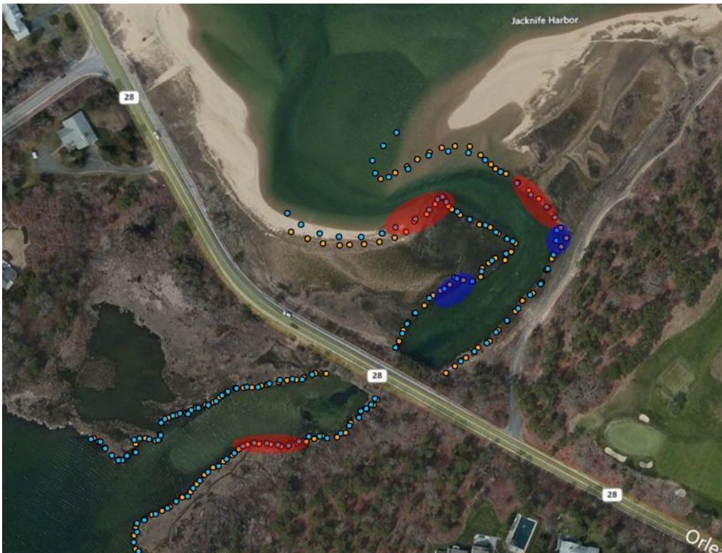
Figure 8. Minor bank slumping has been noted over the monitoring period. Areas of bank slumping are shown in red. Blue areas represent marsh plain that was lower than the adjacent marsh plain prior to construction but have not exhibited significant bank slumping (Applied Coastal Research and Engineering, 2016)
