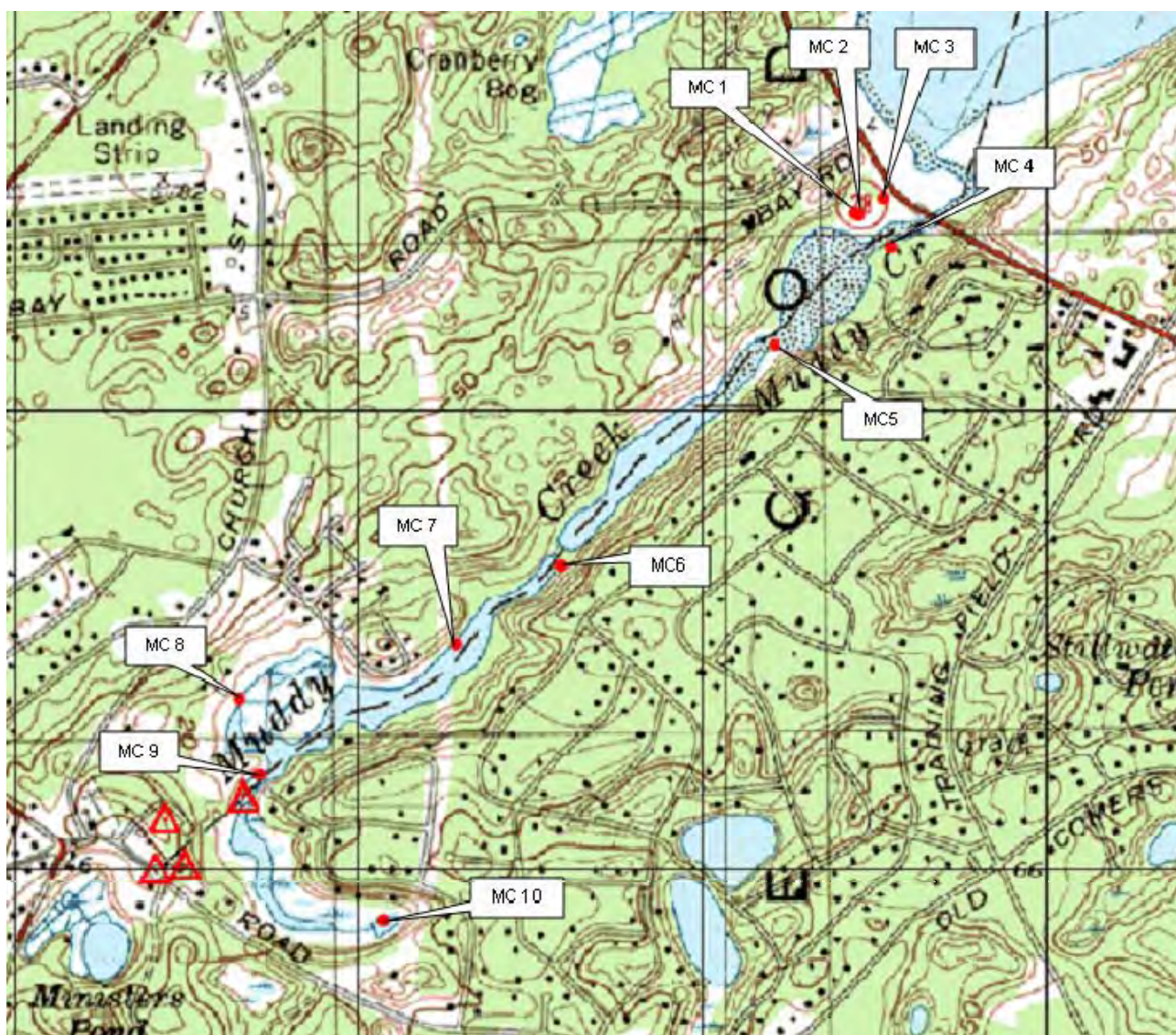
Figure 4 Locations of sediment core sites (red dots labeled MC 10) for determining porewater salinities of wetland areas within the Muddy Creek System. Red triangles show locations of benchmarks.
