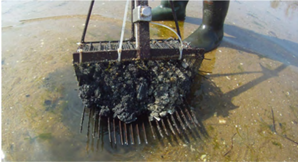
Figure 12 - Modified 1-cubic foot Bullrake for Shellfish Sampling
