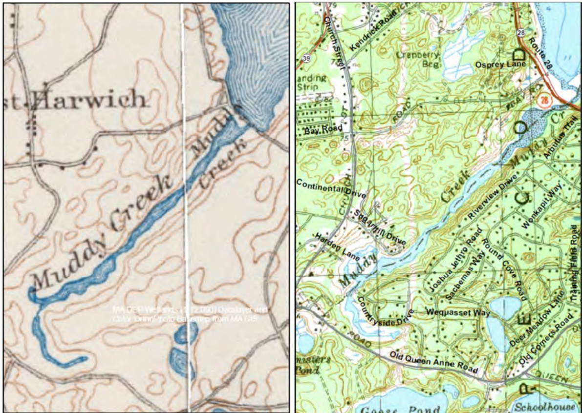
Figure 3 - Comparison of Hydrologic Modifications by Development between the 1890s (left image) and 1960s (right image).
