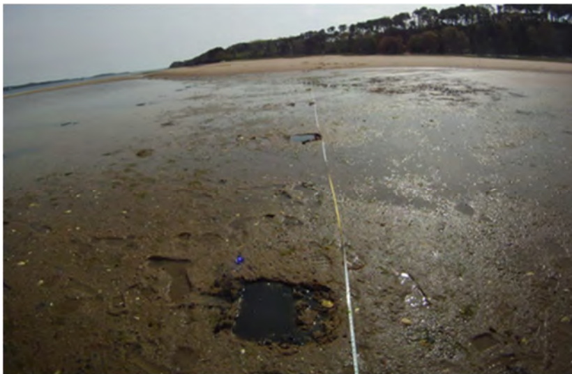
Figure 13 - Typical Layout of Transect Line Sampled at 10-ft Intervals
