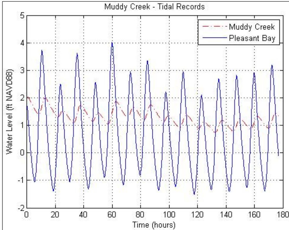
Figure 22. Tide gage records from November 2009 (pre-construction) upstream and downstream of the Route 28 culvert. In 2009, Pleasant Bay was connected to Muddy Creek through a pair of stone box culverts approximately 2.5-foot wide, 3.75-foot in height, and 100-foot in length.
