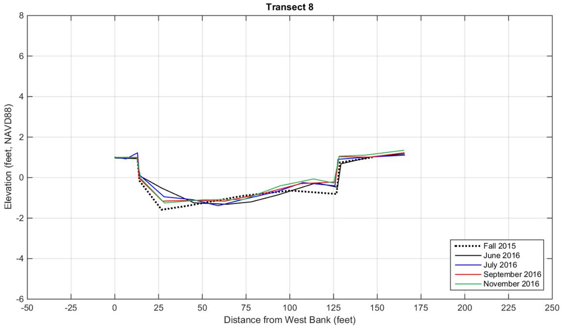
Figure 17. Cross-channel monitoring Transect 8. Distance are relative to the West Channel Bank and datum elevations are given relative to NAVD88.
