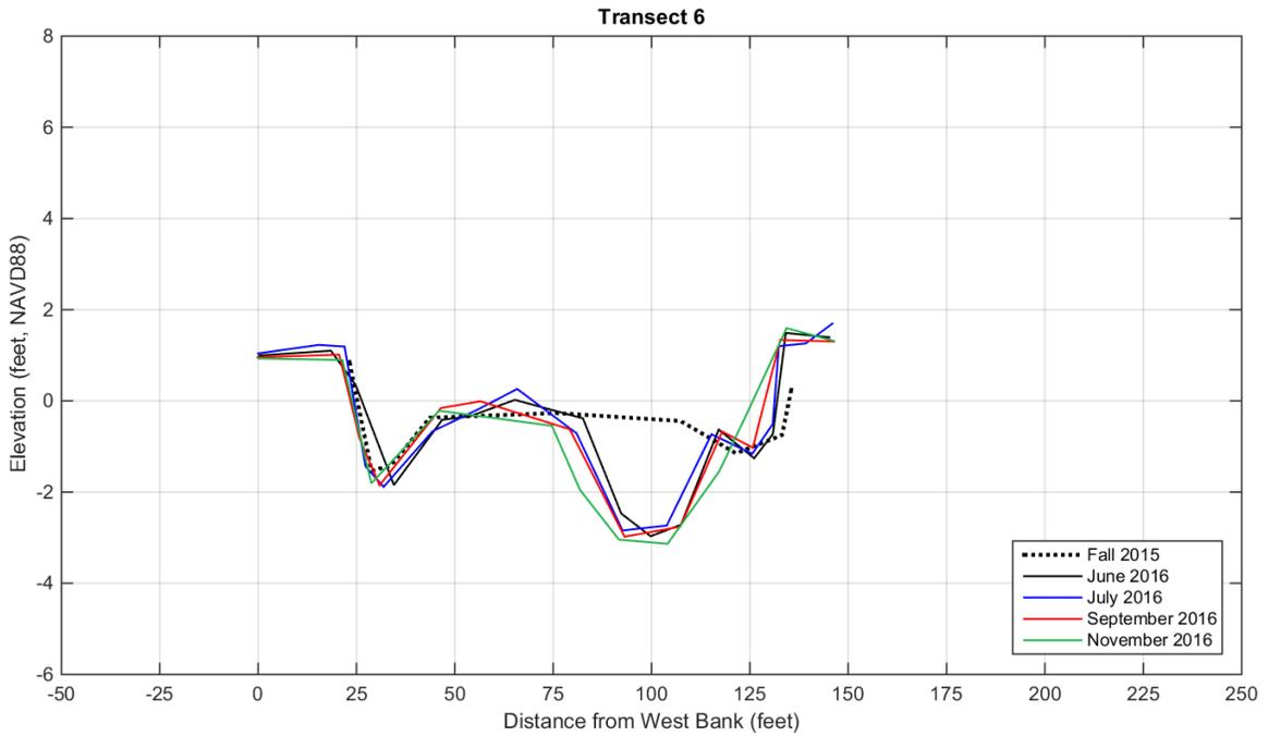
Figure 15. Cross-channel monitoring Transect 6. Distance are relative to the West Channel Bank and datum elevations are given relative to NAVD88.
