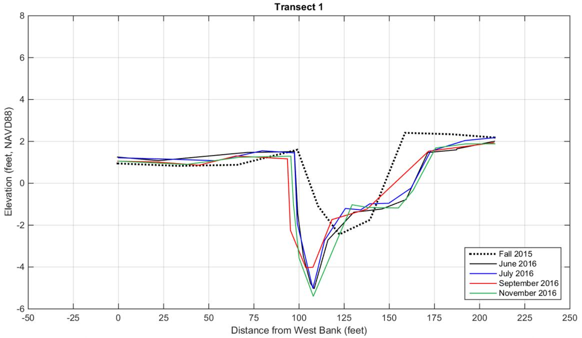
Figure 8. Cross-channel monitoring Transect 1. Distance are relative to the West Channel Bank and datum elevations are given relative to NAVD88.
