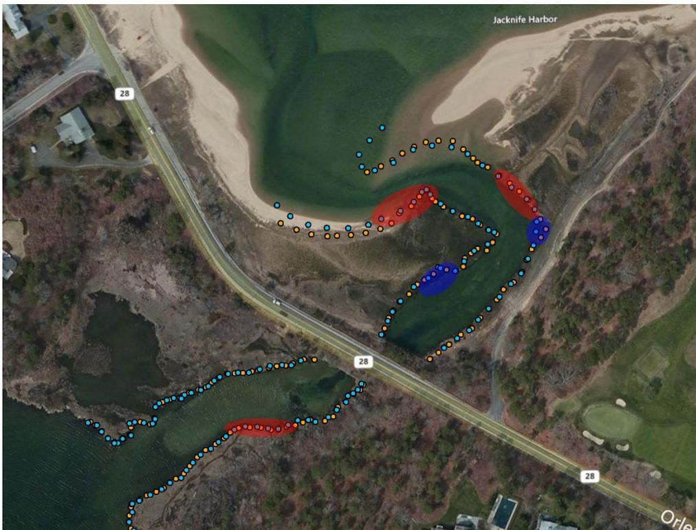
Figure 6. Red areas represent areas where bank erosion has been noted over the monitoring period. Blue areas represent marsh plain that was lower than the adjacent marsh plain prior to construction but have not exhibit significant bank erosion.
