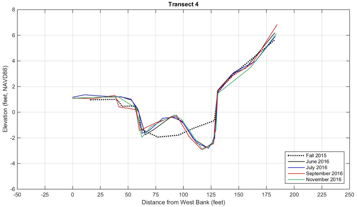
Figure 12. Cross-channel monitoring Transect 4. Distance are relative to the West Channel Bank and datum elevations are given relative to NAVD88.
