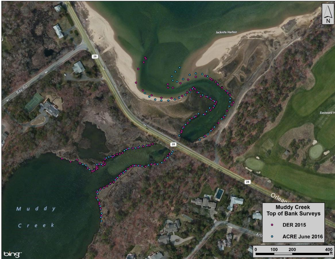
Figure 1. Fall of 2015 (pre-construction) and June of 2016 (post-construction) measured top of bank positions. The measurements are overlaid on a composite 2014 aerial photograph (Bing, 2014) of Muddy Creek. Pleasant Bay is seen in the upper portion of the photo.
