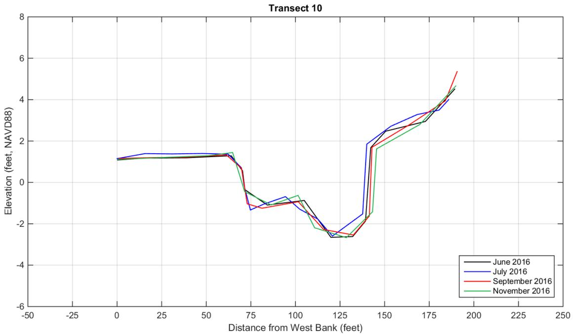
Figure 11. Cross-channel monitoring Transect 10. Distance are relative to the West Channel Bank and datum elevations are given relative to NAVD88.
