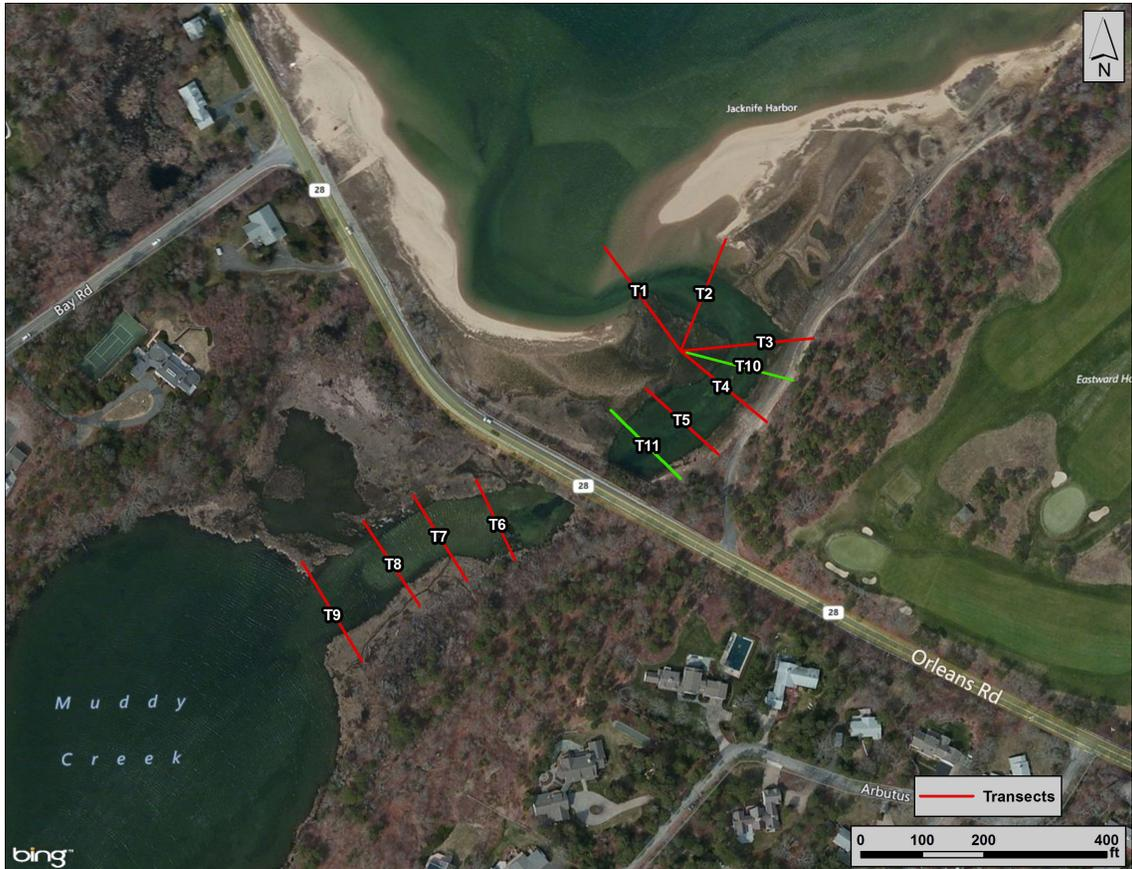
Figure 7. Locations of the cross-channel monitoring transects. Two additional transects were added to the post-construction monitoring, Transects 10 and 11, which are highlighted in green.
