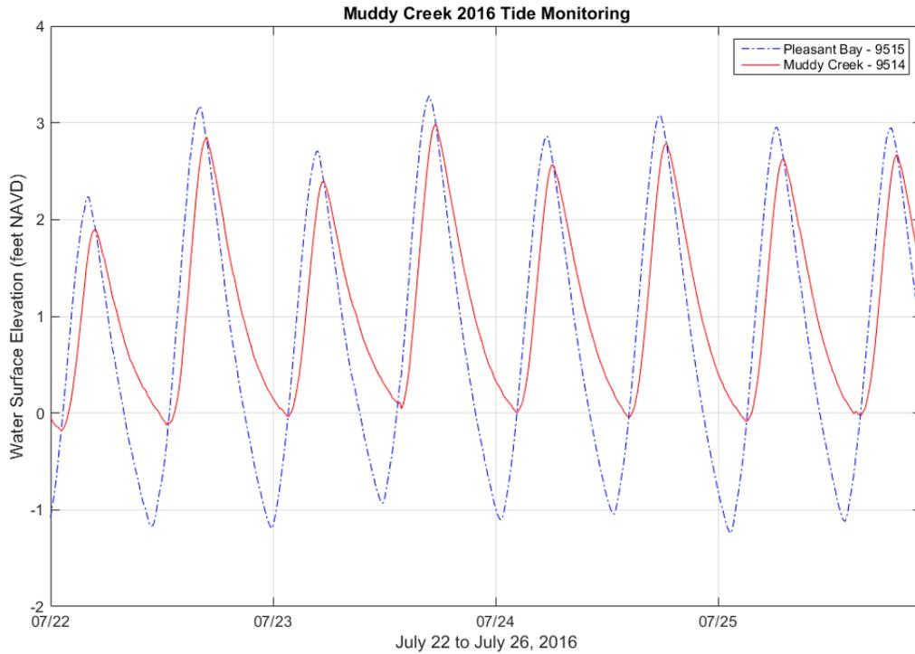
Figure 21. Plot showing three tide cycles in Pleasant Bay and upstream of the new Route 28 Bridge in Muddy Creek.
