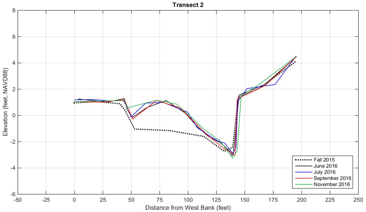
Figure 9. Cross-channel monitoring Transect 2. Distance are relative to the West Channel Bank and datum elevations are given relative to NAVD88.
