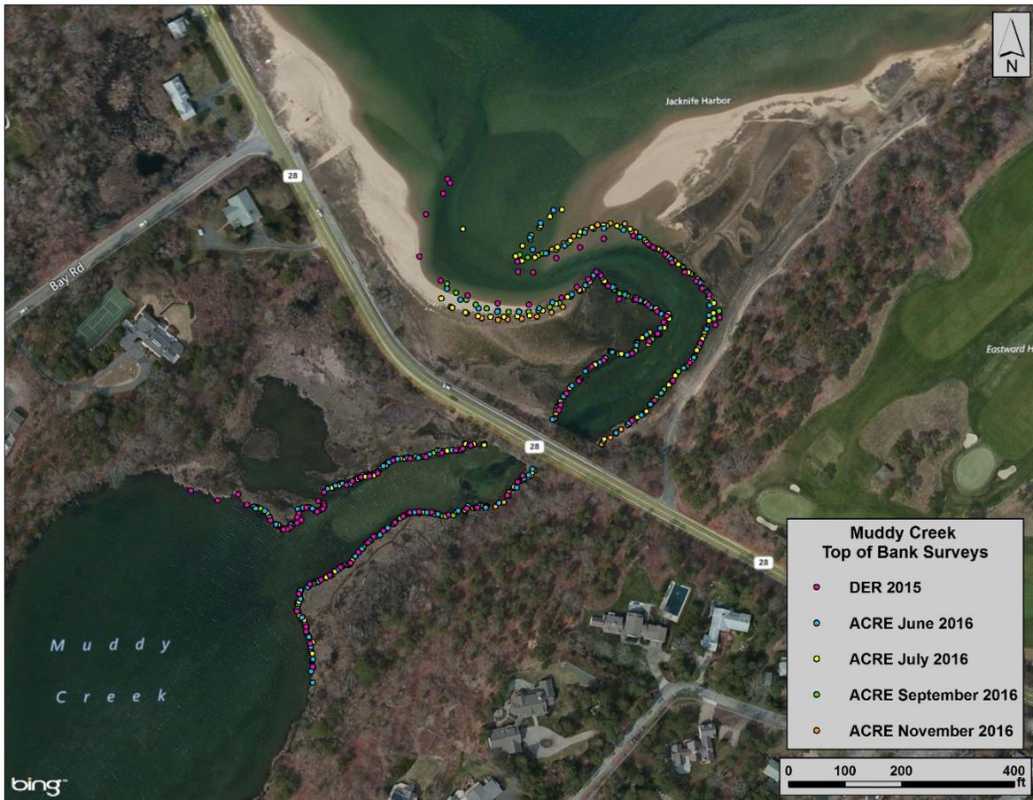
Figure 4. Composite of all the measured top of bank positions. The measurements are overlaid on a composite 2014 aerial photograph (Bing, 2014) of Muddy Creek. Pleasant Bay is seen in the upper portion of the photo.
