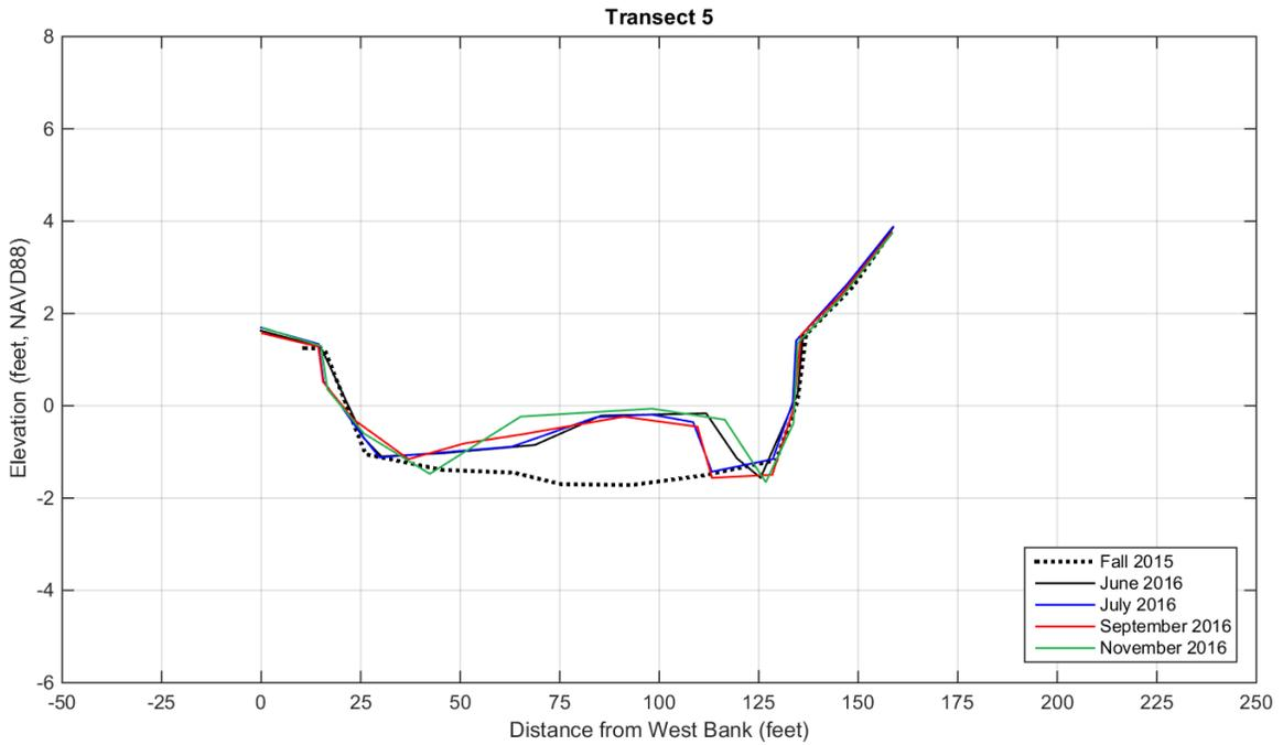
Figure 13. Cross-channel monitoring Transect 5. Distance are relative to the West Channel Bank and datum elevations are given relative to NAVD88.
