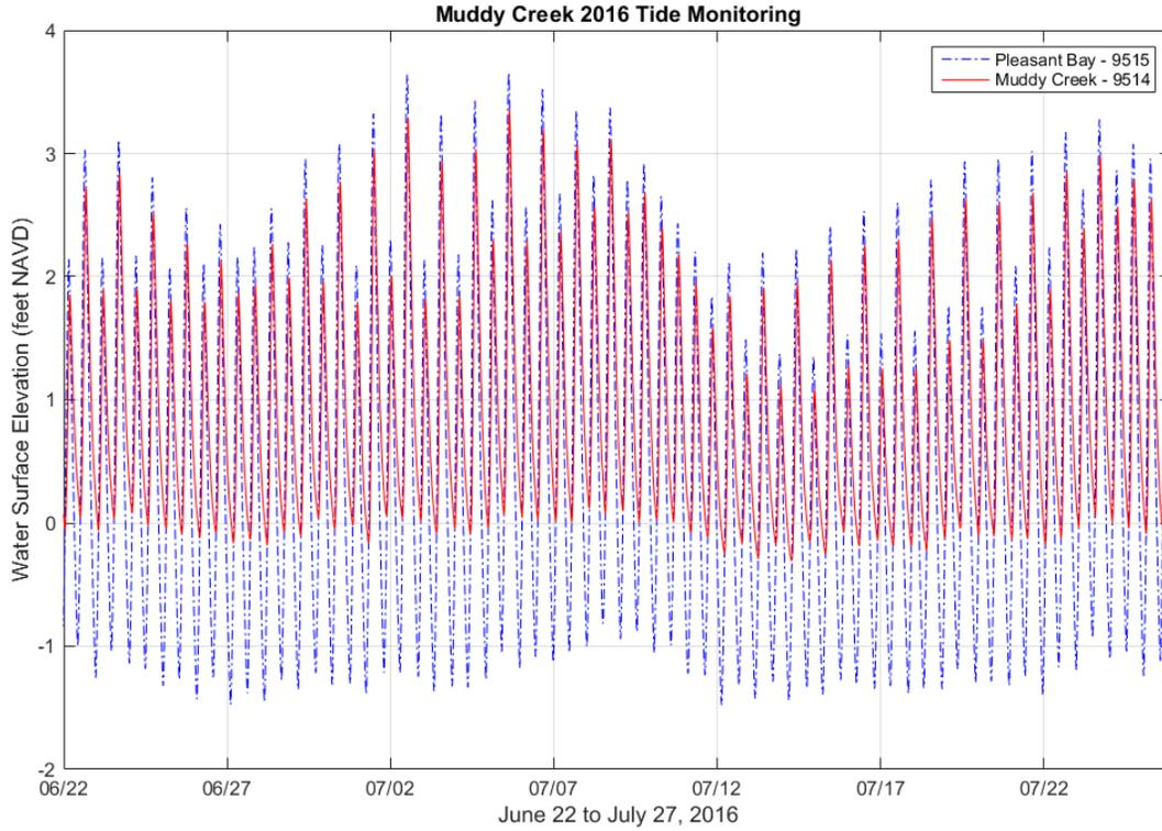
Figure 20. Plots of observed tides for the Muddy Creek, Chatham and Harwich, MA, for the 34-day period between June 1, 2016 and July 16, 2016. The blue line shows tide offshore in Pleasant Bay. The red line shows the tide inside Muddy Creek upstream of the new Route 28 Bridge. All water levels are referenced to the NAVD 88.
