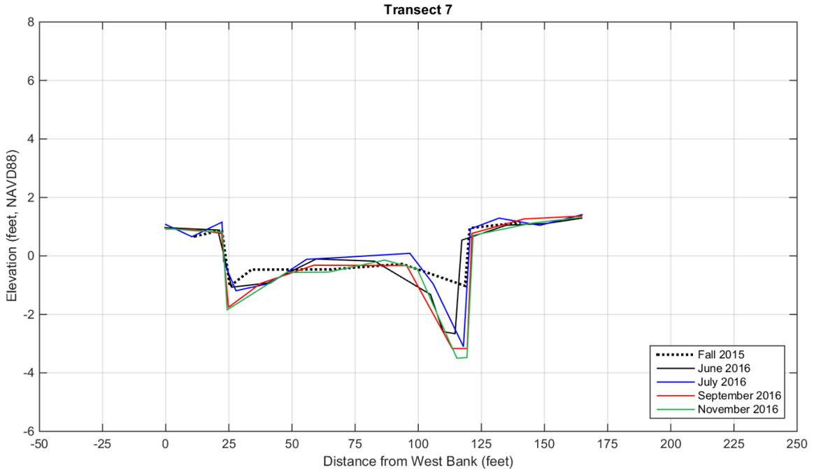
Figure 16. Cross-channel monitoring Transect 7. Distance are relative to the West Channel Bank and datum elevations are given relative to NAVD88.
