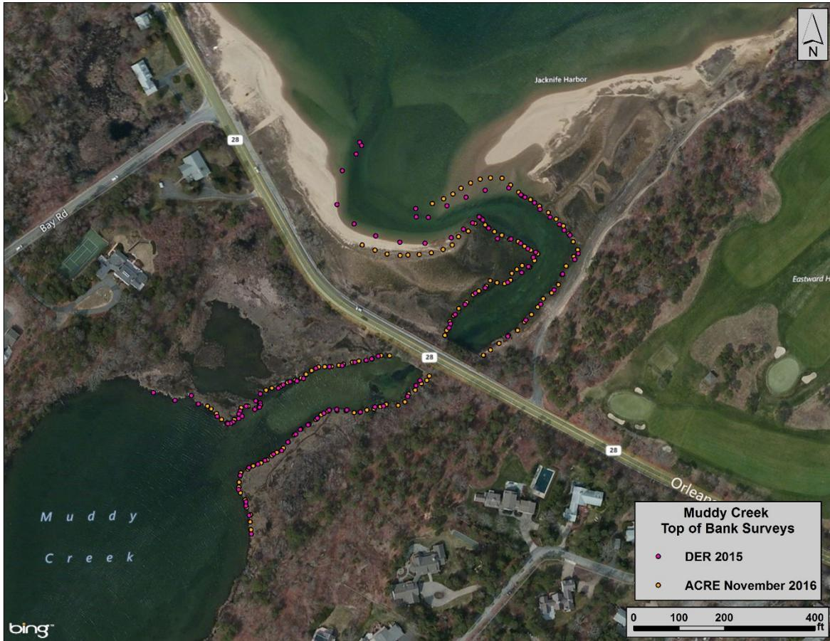
Figure 2. Fall of 2015 (pre-construction) and November of 2016 (post-construction) measured top of bank positions. The measurements are overlaid on a composite 2014 aerial photograph (Bing, 2014) of Muddy Creek. Pleasant Bay is seen in the upper portion of the photo.
