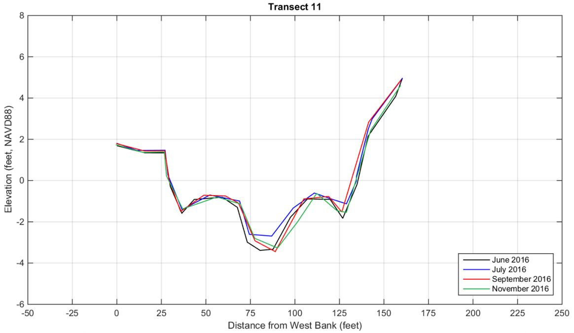
Figure 14. Cross-channel monitoring Transect 11. Distance are relative to the West Channel Bank and datum elevations are given relative to NAVD88.
