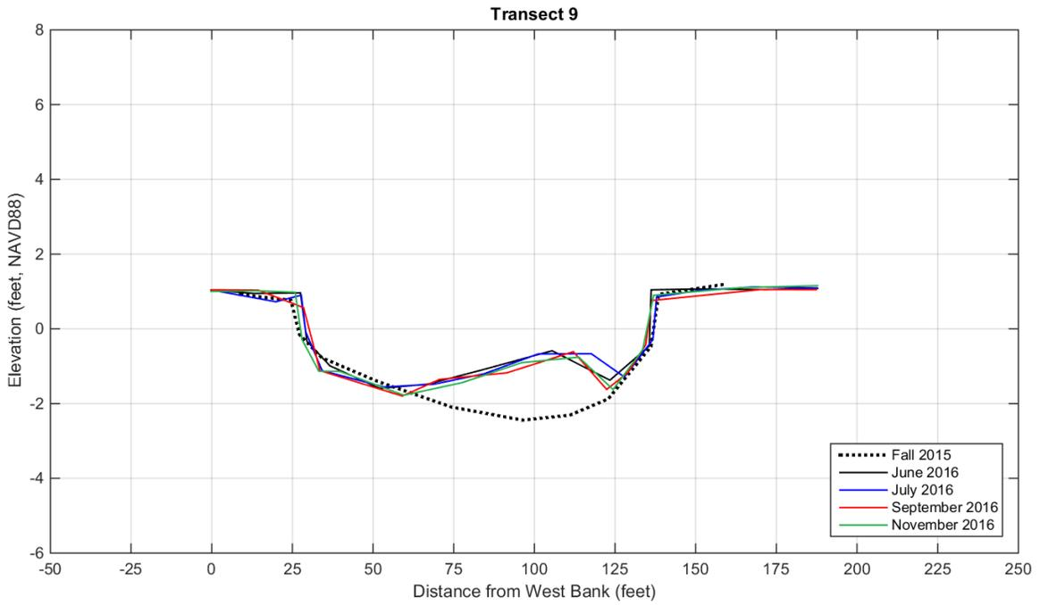
Figure 18. Cross-channel monitoring Transect 9. Distance are relative to the West Channel Bank and datum elevations are given relative to NAVD88.
