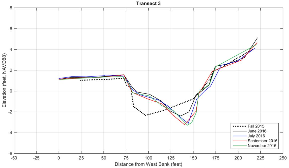
Figure 10. Cross-channel monitoring Transect 3. Distance are relative to the West Channel Bank and datum elevations are given relative to NAVD88.
