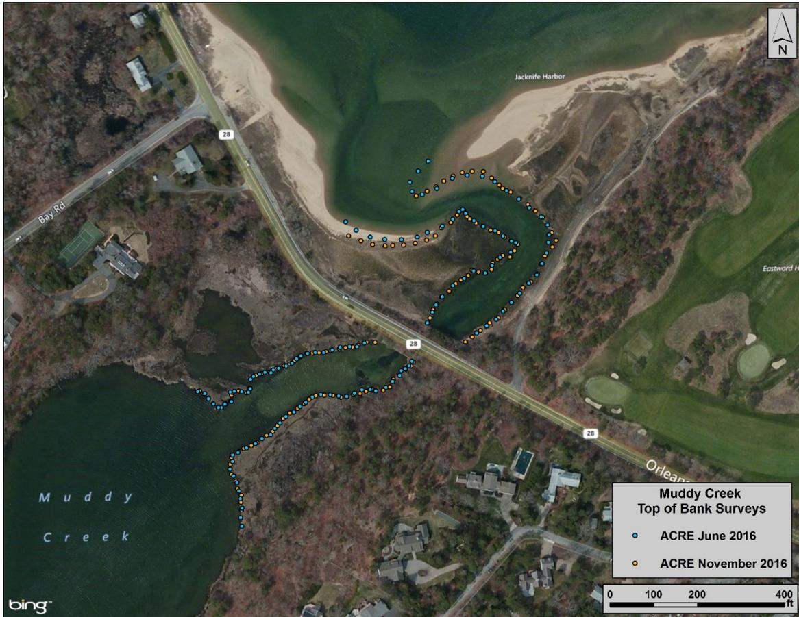
Figure 3. June of 2016 and November of 2016 measured top of bank positions. The measurements are overlaid on a composite 2014 aerial photograph (Bing, 2014) of Muddy Creek. Pleasant Bay is seen in the upper portion of the photo.
