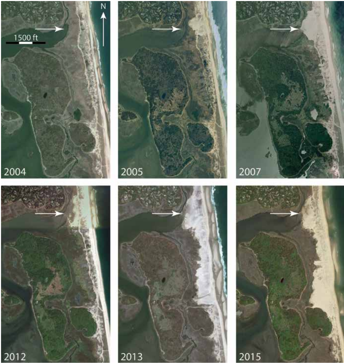
Figure 10. Example of overwash events at Pochet Island. The white arrow is provided to reference change in washover fan through time. This is also one of the ways that barrier islands keep pace with sea level rise. When overwash occurs the island increases in elevation in that area.
