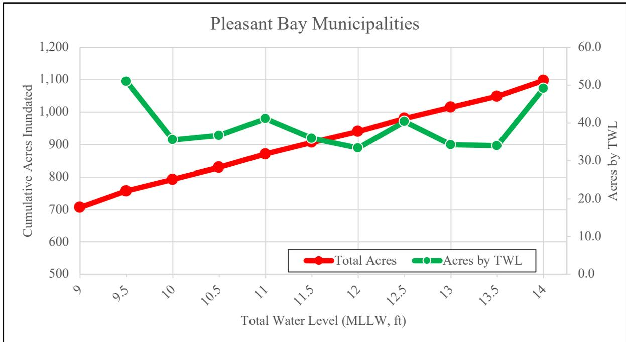
Figure 6. The red line represents the total cumulative area inundated with each 6-inch increase in total water level. The green bars represent the area inundated for each individual 6-inch increase in total water level. The average is approximately 450 acres per 6-inch increase in total water level.
