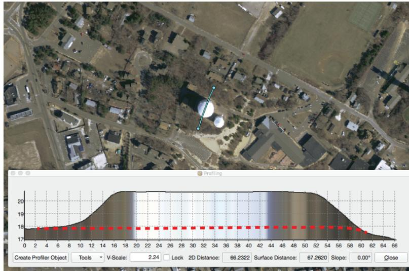
Figure 2. Example of ‘pull up’ near a water tower in Provincetown. Dotted red line is more representative of elevations at the water tower. Blue line in image is location in profile. Profile units = meters (Vert. NAVD88, Hor. NAD83), image taken from Borrelli, et al., 2017.
