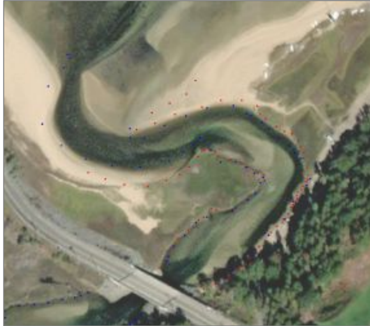
Figure 3.2 Measured bank position in 2015 (blue markers) and 2021 (red markers).
