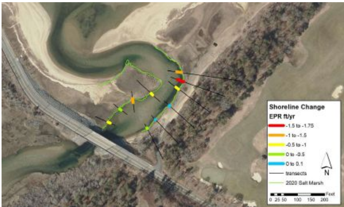
Figure 3.3 Shoreline erosion rates along the inlet channel to Muddy Creek between 2016 and 2020.
