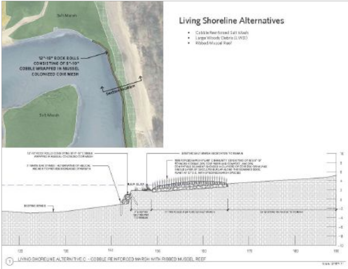
Figure 4.8 Typical cross-section of a Cobble Reinforced Marsh with ribbed mussel reef.
